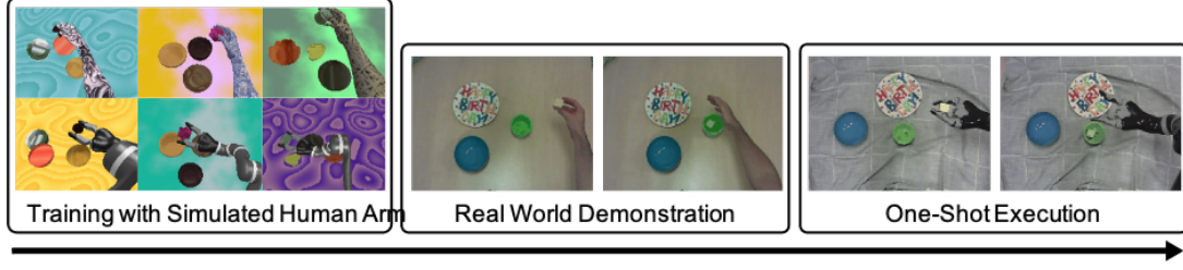
Figure 5.9: The robot gains its ability to infer actions from humans in simulation, and can then learn a new task from a single human demonstration in the real-world.
