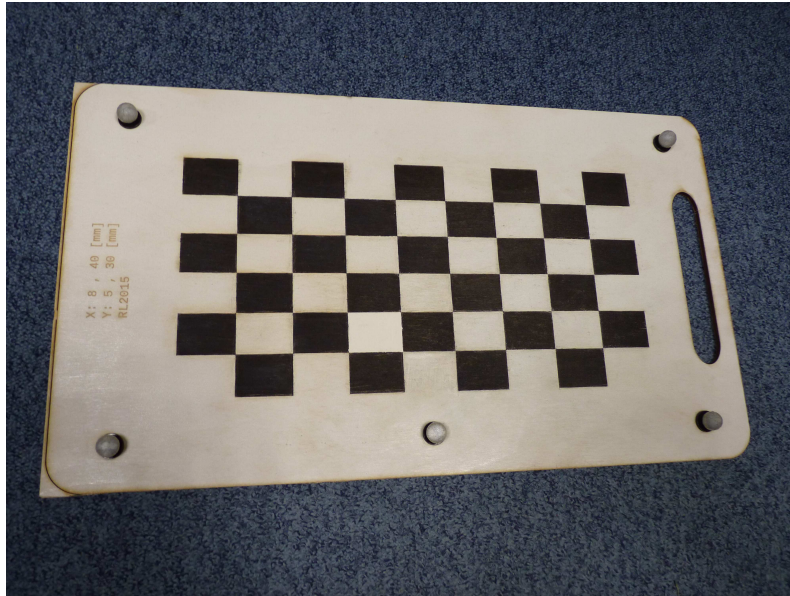
Figure 2.8: Combined vision and ground truth tracker calibration pattern.
