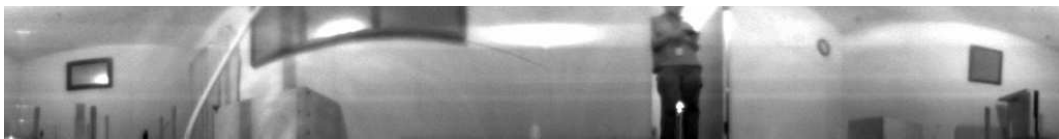
Figure 3.2: Optical artifacts from a low-cost omnidirectional lens.
