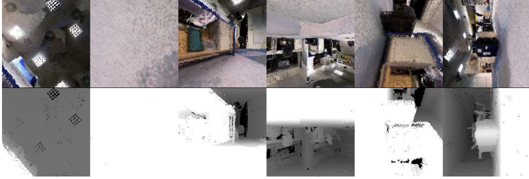
Figure 2.10: Scene rendered 6 times to produce a cube map.
