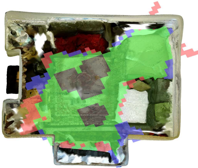
Figure 6.36: Dataset “Wandsworth Livingroom”, 3D model with occupancy grid overlay.
